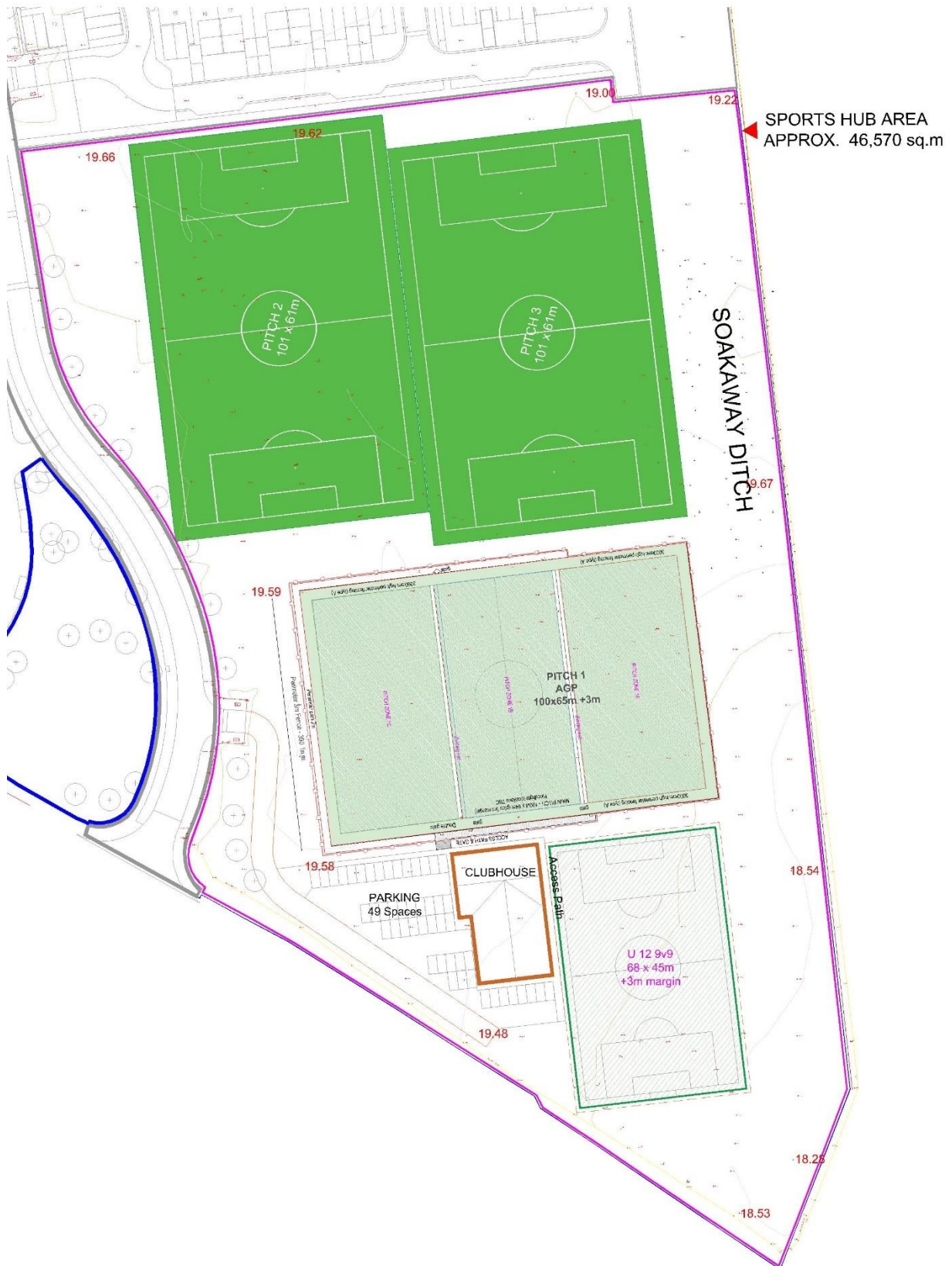
Fig 17. Layout option 2 – for grass and full-sized 3G AGP, the senior sized pitches could be ‘subdivided’ for junior pitch layouts with alternative line-marking
