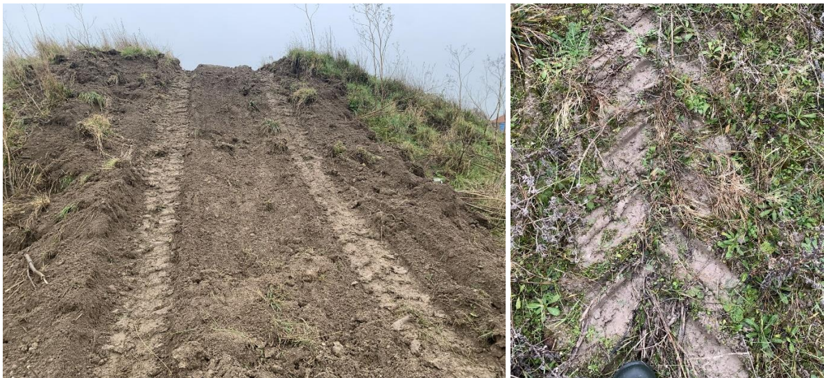
Fig 7. Left – Mound ‘K’ appears to be mostly topsoil. Right – The soil does compact and smear under trafficking when wet.
