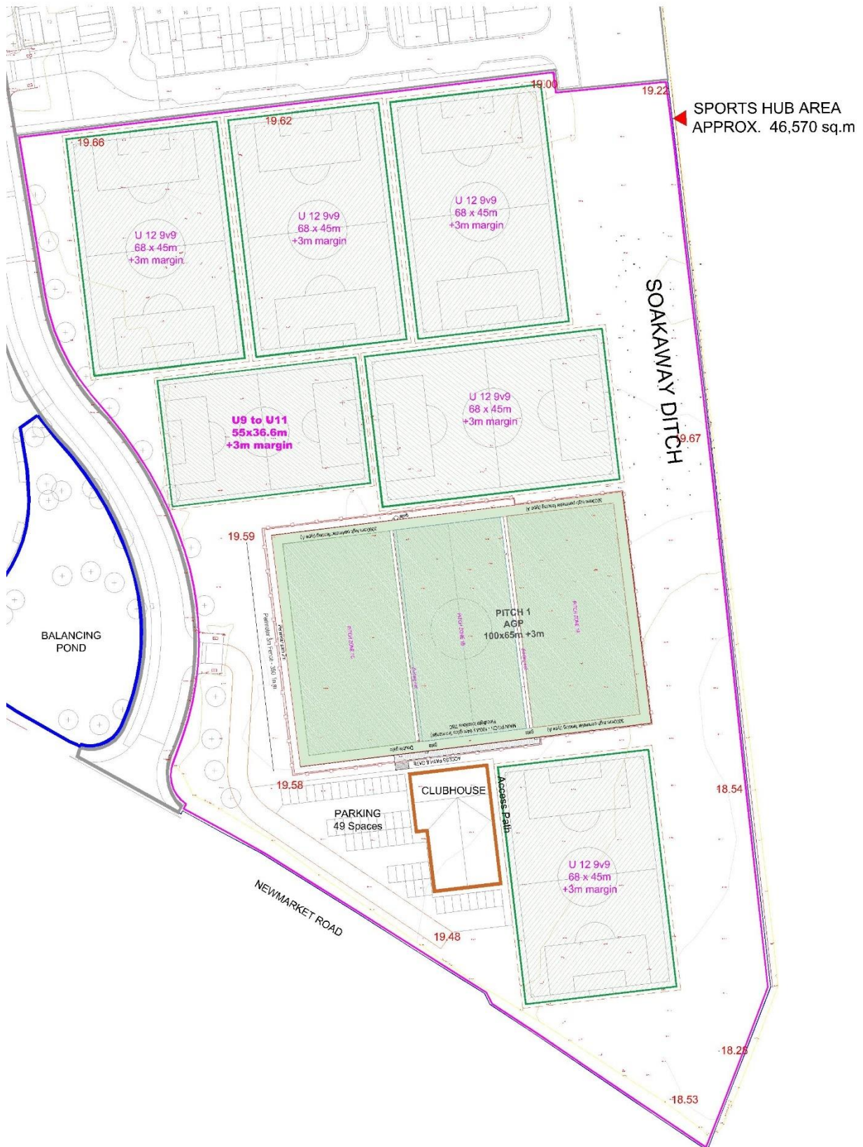
Fig 18. Layout option 3 – for grass and full-sized 3G AGP, with junior pitch options.
