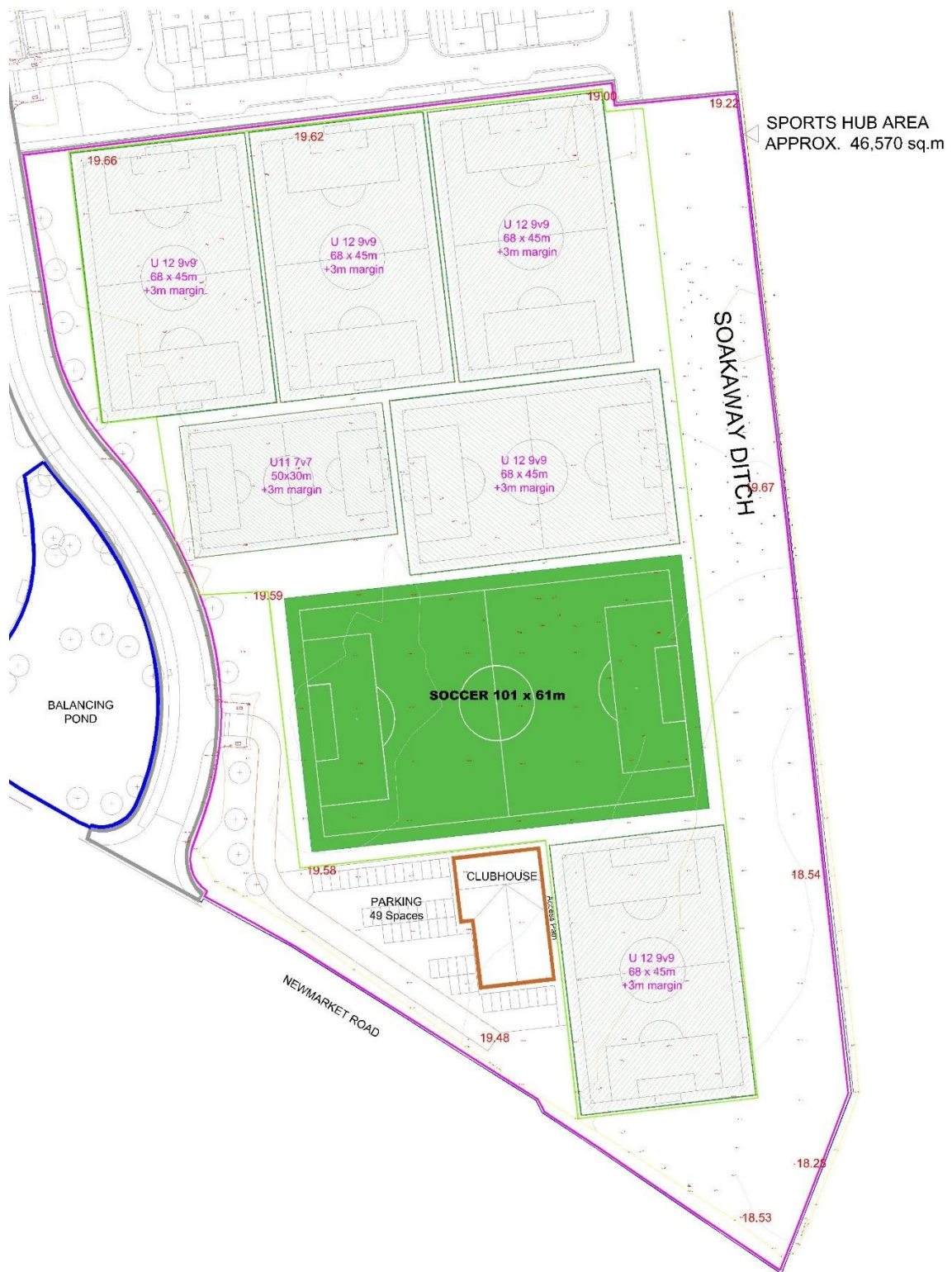
Fig 16. Layout option 1 – for grass only pitches, one first team pitch plus junior pitches – there are many connotations for line-marking other pitch size combinations.
