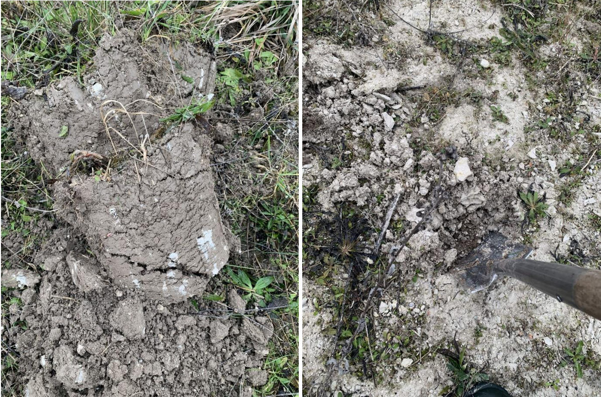
Fig 6. The topsoil overlies a hard chalky subsoil
