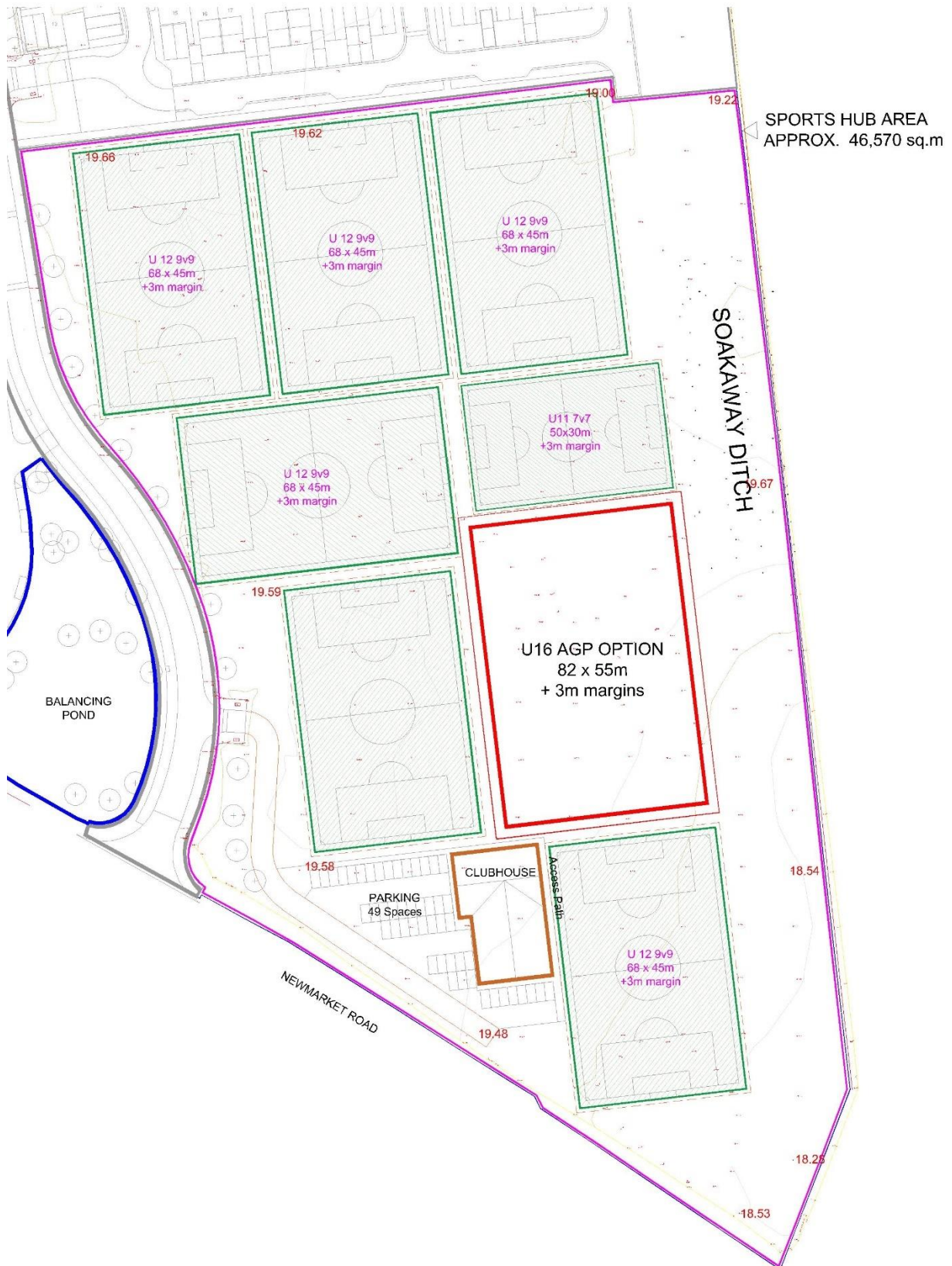
Fig 19. Layout option 4 – for grass and smaller sized 3G AGP, with junior pitch options.
